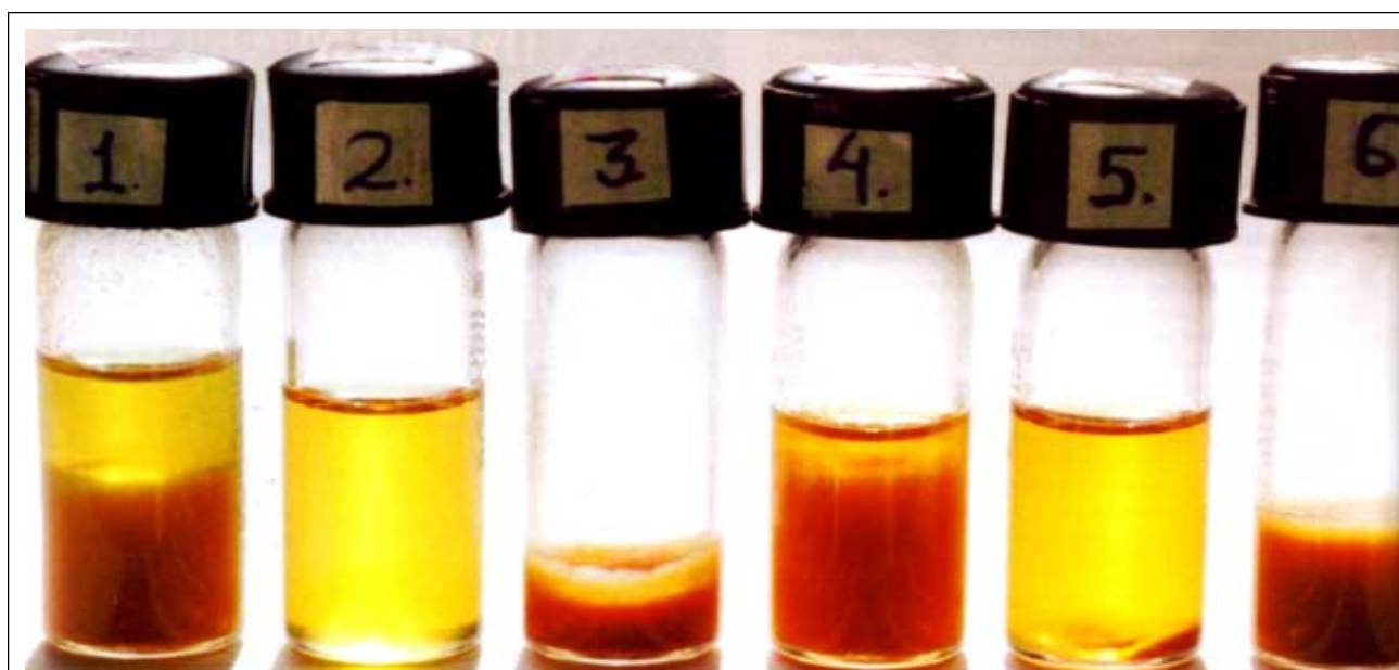
Fig. 1. Photograph illustrating neat crude oil extraction from rice bran at 5°C. (1) Hexane extract (normal extraction); (2) hexane extract at 5°C; (3) hexane extract (normal extraction of residual bran) (from 5°C extracted spent rice bran); (4) acetone extract (normal extraction); (5) acetone extract at 5°C; (6) acetone extract (normal extraction of residual bran) (from spent rice bran). Source: Gopala Krishna et al., 2011
