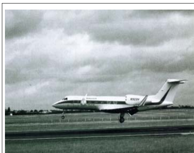
FIG. 1. The Gulfstream G450jet lands in Paris, France, after flying from New Jersey, USA, on a 50:50 blend of camelina oil-based and petroleum-based jet fuels. Courtesy of Honeywell Aerospace
