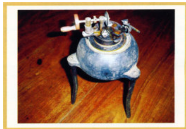
Figure 6 : Flash point apparatus
