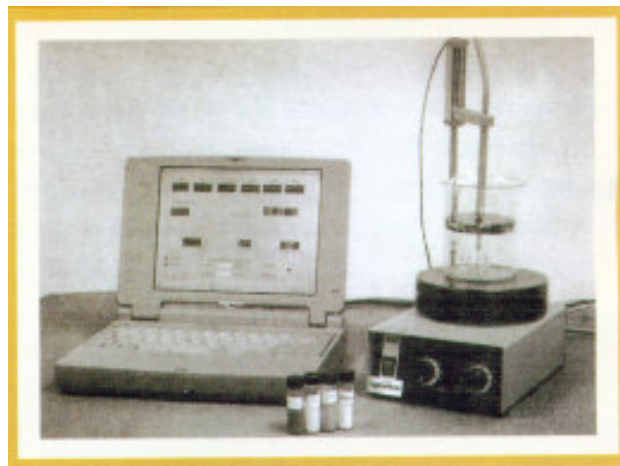
Figure 2: Automatic apparatus for slip melting point ;
