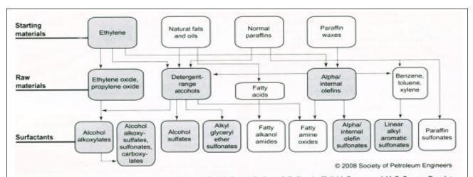
FIG. 1. Different routes to surfactants. Source: Barnes, J.R., J.P. Smit, J.R. Smit, P.G. Shpakoff, K.H. Raney, and M.C. Puerto, Development of Surfactants for Chemical Flooding at Difficult Reservoir Conditions, Paper SPE-113313-MS, presented at the Society of Petroleum Engineers/Department of Energy Improved Oil Recovery Symposium, Tulsa, Oklahoma, USA, April 19–23, 2008. Shaded boxes: Shell Chemical commercial routes and surfactants
