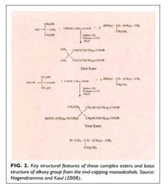
polyol, diearboxylie acid, and nonoalcohol as an end-capping agent. Key structural features of these esters and the basic structure of the alkoxy group from the end-capping monoaleohols are presented in Figure 2.
